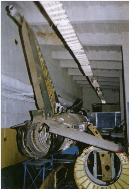
Yet another cutaway Ye-2A, this time at an aviation technical school in Moscow. The red-painted areas on the stabilator are 'mind your head' caution markings for the students. The ejection seat headres bears the stencil 0632 – that is, izdeliye 63 No. 2.
