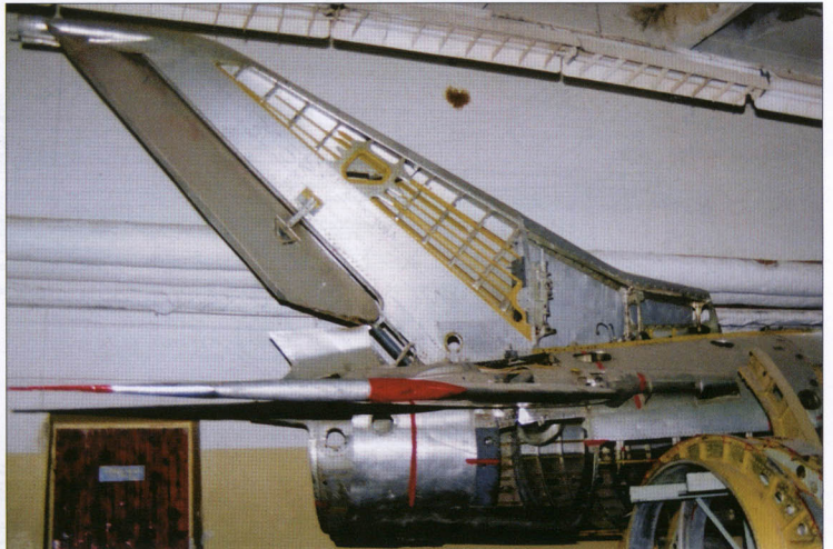
Yet another cutaway Ye-2A, this time at an aviation technical school in Moscow. The red-painted areas on the stabilator are 'mind your head' caution markings for the students. The ejection seat headres bears the stencil 0632 – that is, izdeliye 63 No. 2.
